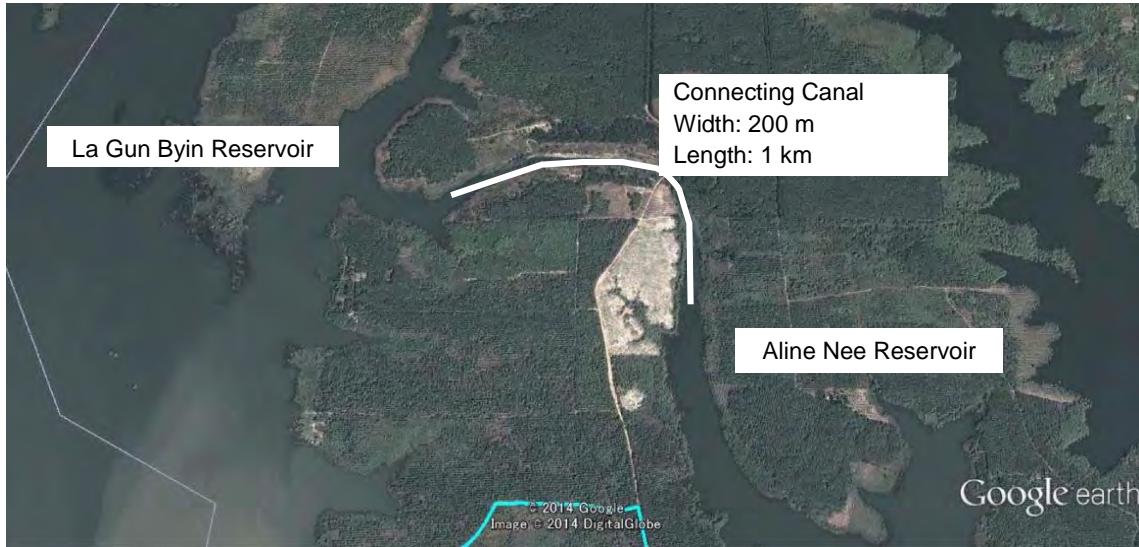
Figure 6-3-4 Location of Connecting Canal
