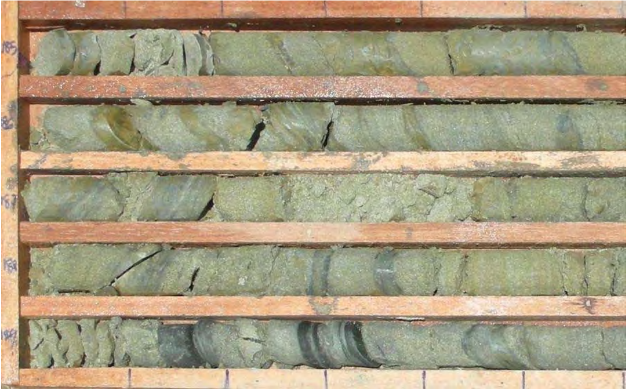
Figure 3-2-5-12 D-2 186.0 ~ 189.5 m - Weakly Consolidated Sandstone (Crushable with Fingers)
