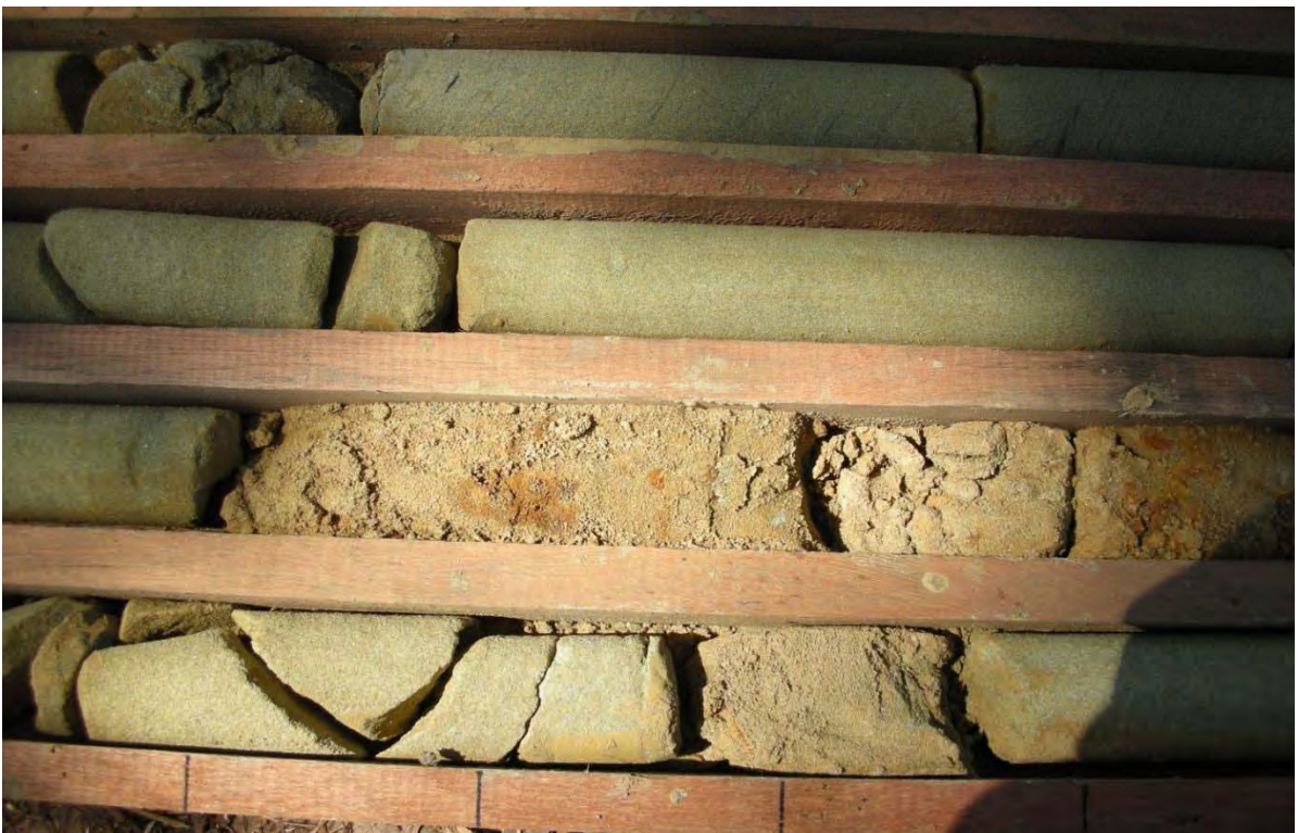
Figure 3-2-5-11 D-2 131.5 ~134.5 m-Hard Sandstone and Brownish Weakly Consolidated Sandstone
