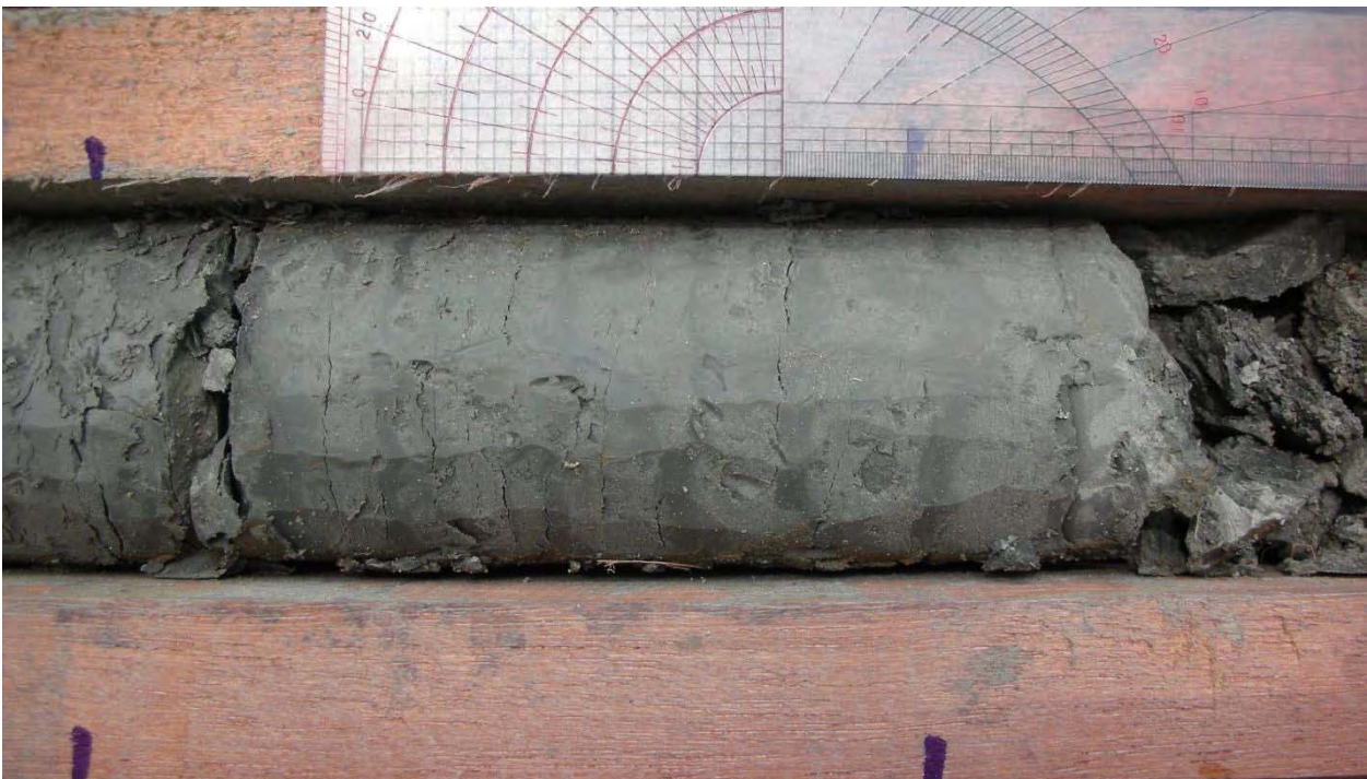
Figure 3-2-5-13 D-2 249.4 ~ 249.55 m - Fine Alternation of Clay and Silt; Almost Horizontally Bedded
