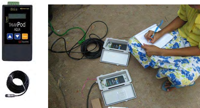
Figure 3-2-13-4 Automatic Water Level Meter used for the Test
