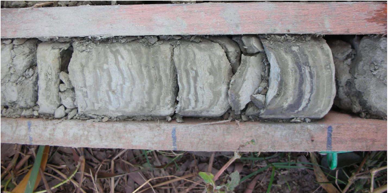
Figure 3-2-5-15 D-4 9.3 ~ 9.5 m - Fine Alternation of Silt and Very Fine Sand (Disturbed by Drilling Torque)
