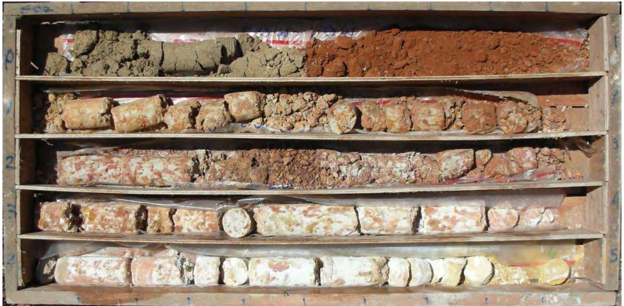
Figure 3-2-5-8 D-2 Surface - Lateritic Soil and Weathered Zone
