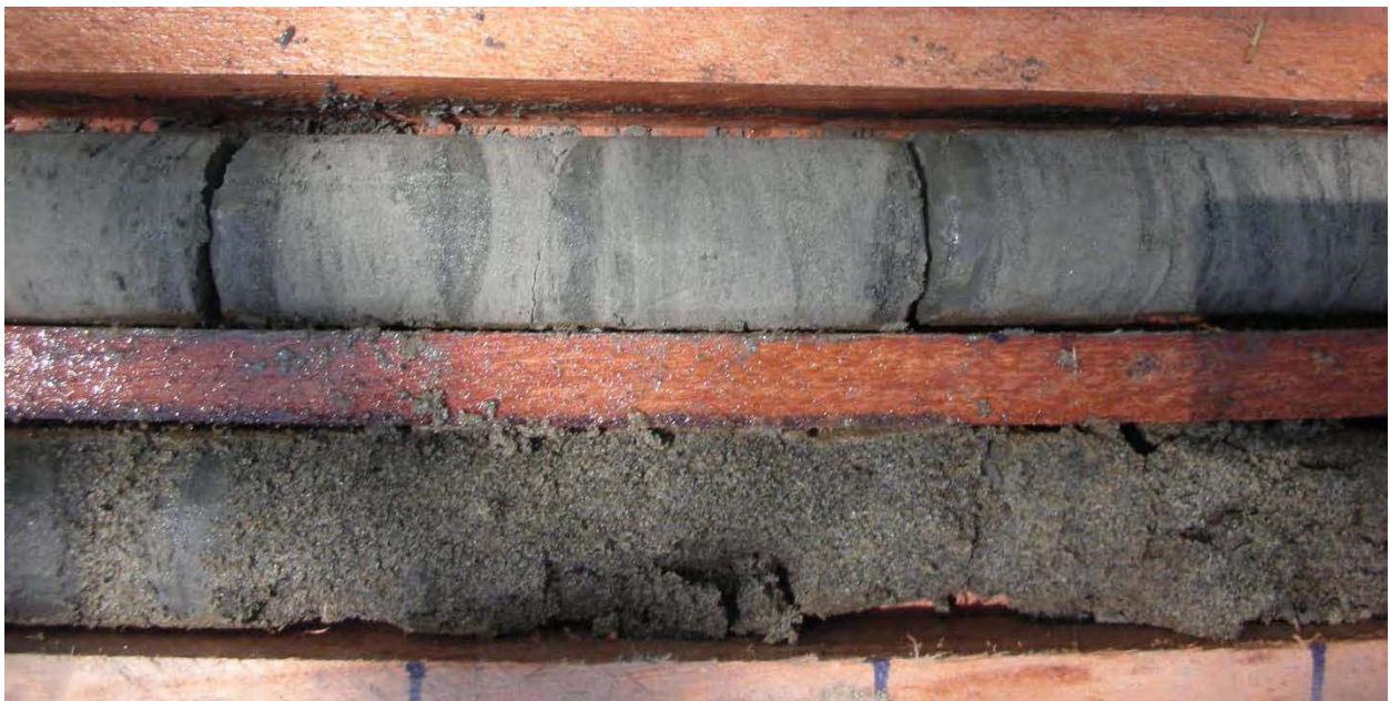
Figure 3-2-5-19 D-4 223.5 ~ 224.5 m - Alternation of Silt and Very Fine Sand, and Slightly Consolidated Sandstone
