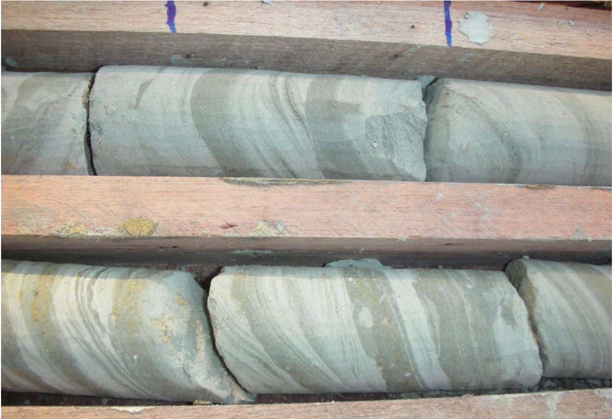
Figure 3-2-5-10 D-2 95.5 ~ 96.5 m - Semi-consolidated Fine Alternation of Silt and Very Fine Sand
