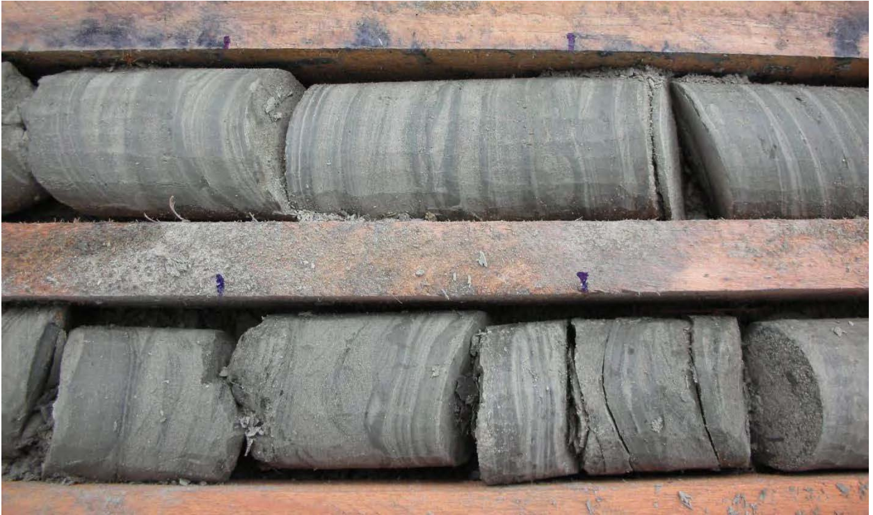
Figure 3-2-5-14 D-2 255.5 ~ 256.5 m - Fine Alternation of Silt and Very Fine Sand; Dipping Approx. 15°
