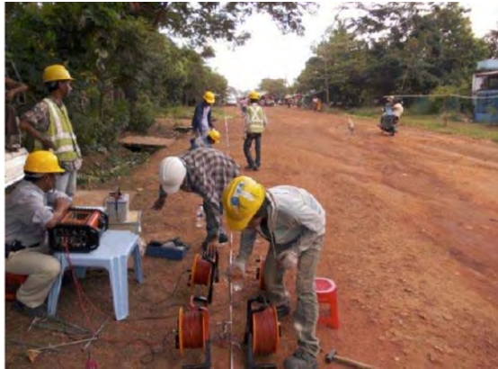
Field survey of VES (Geophysical prospecting) (October 2012)
