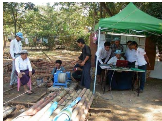
Geophysical logging of test well (D5 site) (January 2013)
