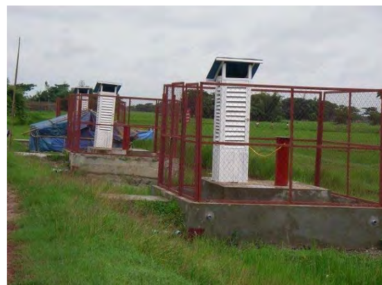
Observation stations of groundwater level of test wells (D-3 site) (October 2013)
