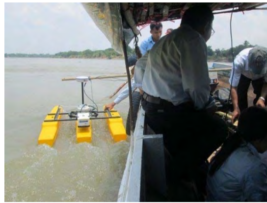
River discharge measurement by ADCP (May 2014)
