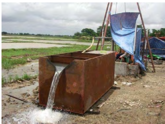
Pumping test of test well (D-3 site) (June 2013)
