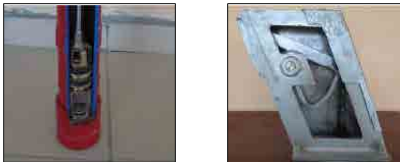
Figure 4.1 Handpump sample for explaining function (left: cylinder of RUWATSAN I right: pump head of RUWATSAN I)
