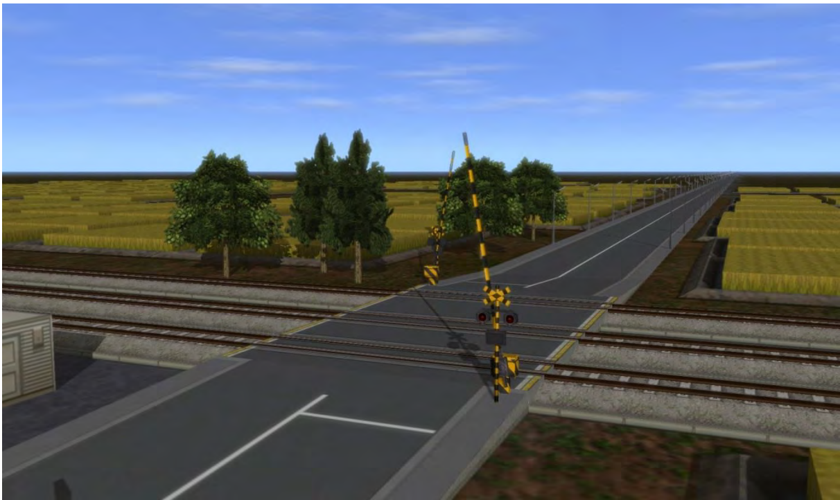
Installation of the automated level crossing alarm facilities between Toegyaungkalay and Ywathagyi completion prospective figure
