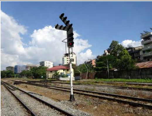
Pic-21: German style signal(LED). The signal which is united with a course indicator.
