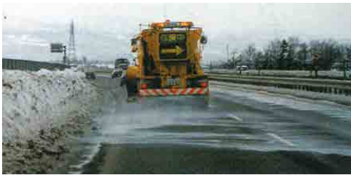
<Figure8-1> Anti-freezing agent spreading in Japan (left) and the conceptual view of anti-freezing agent spray vehicle (right)
