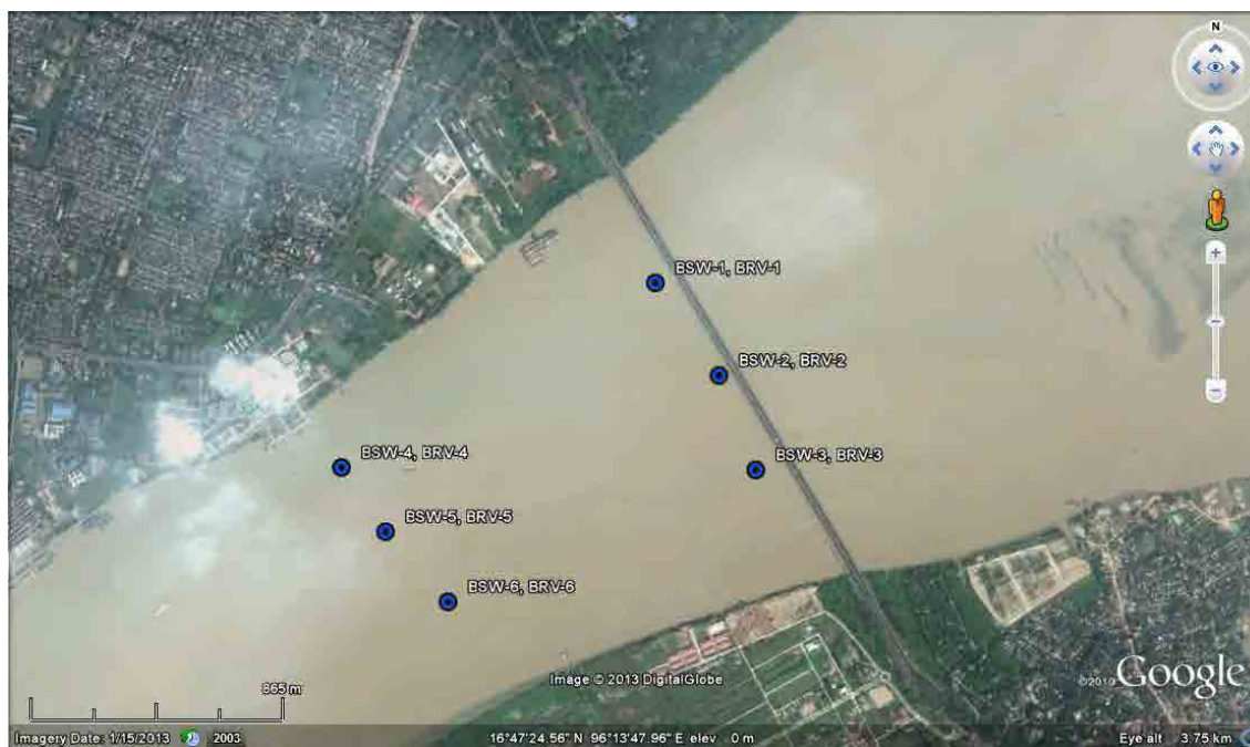
Figure 12.13 Location of Water Sampling and River Velocity Measurement
