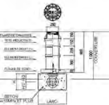
VANNE A PASSAGE DIRECT 100 (COUVERTURE H=1.0m)
