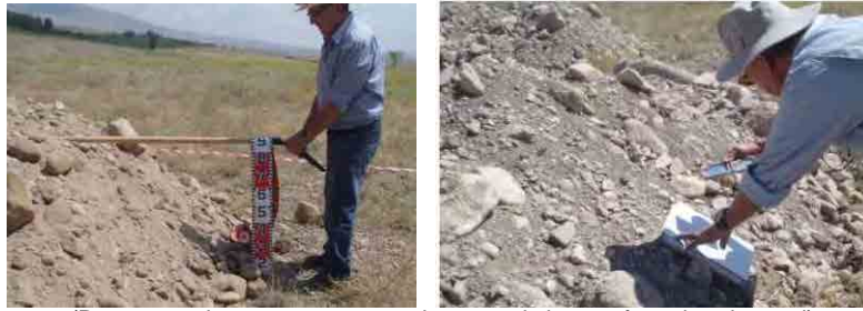
(Repose angle measurement on the natural slopes of sand-and-gravel)
