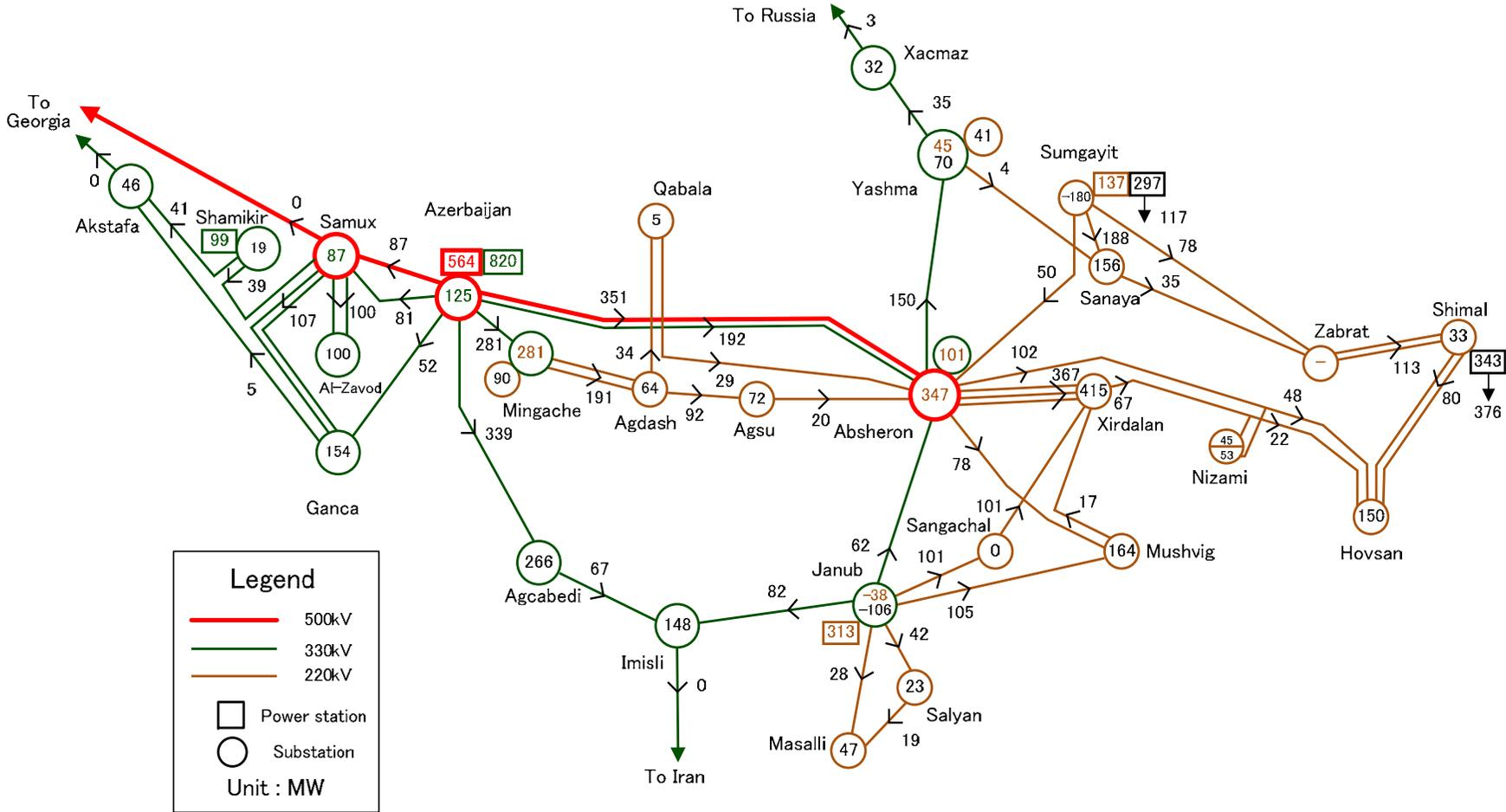
Source: Power flow analysis result by JICA Study Team using digital network analysis data provided from JSCA
