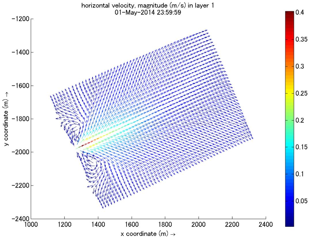
**Figure 13.6-16(3) Flow Condition with Thermal Effluent (Current speed 0m/s)**
