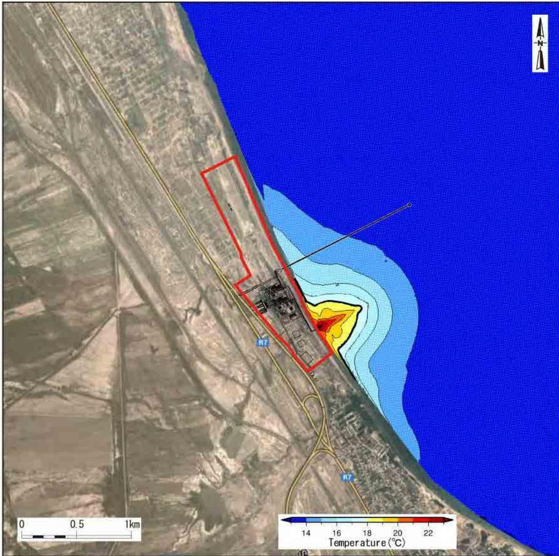
**Figure 13.6-13(2) Dispersion of Thermal Effluent (Current speed 0m/s)**
