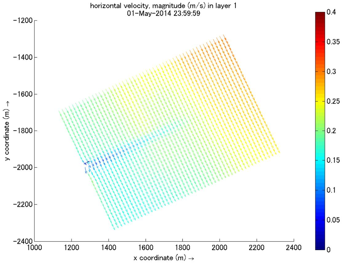
**Figure 13.6-16(1) Flow Condition without Thermal Effluent (The present : Current speed 0.3m/s: SE)**
