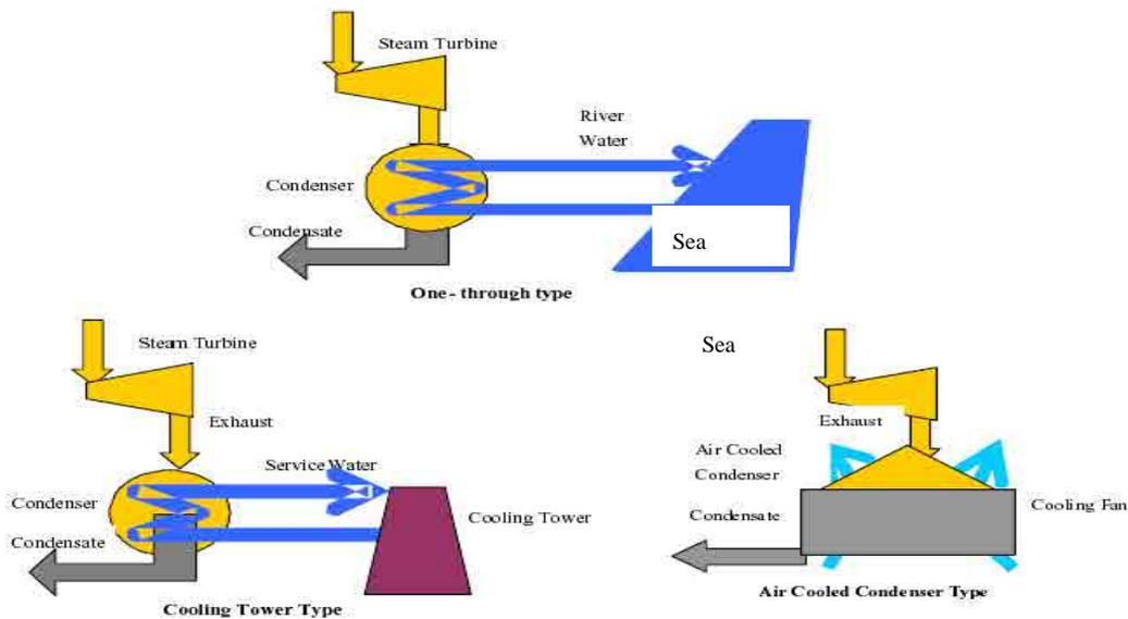
**Figure 13.3-3 Three Method of Cooling System**
