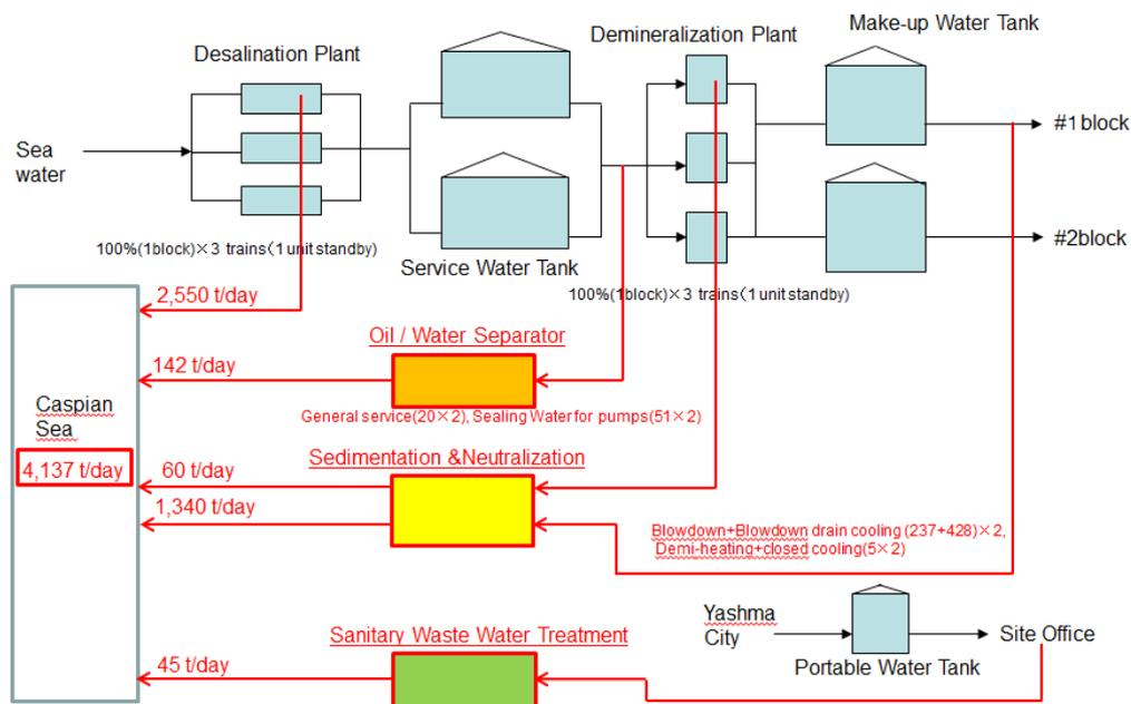
**Figure 13.6-14 Waste Water Flow Diagram**
