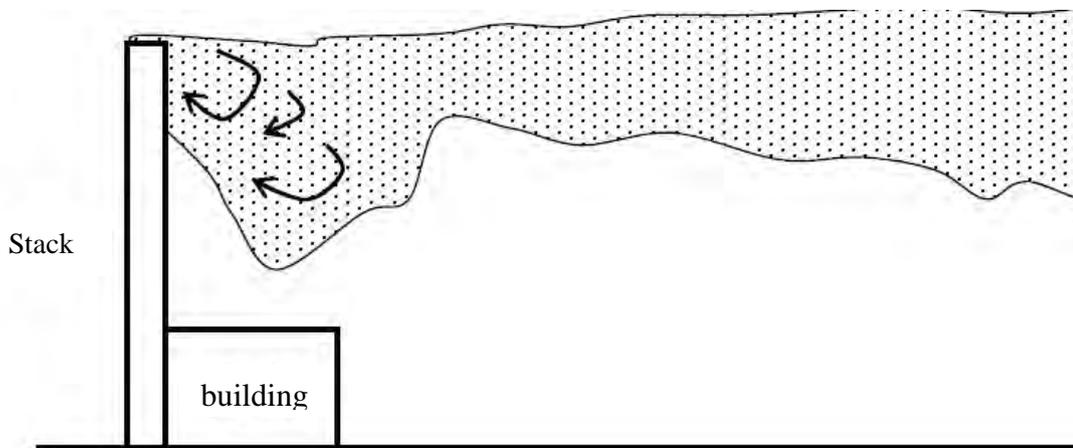
**Figure 13.6-5 Diagram of Downwash**
