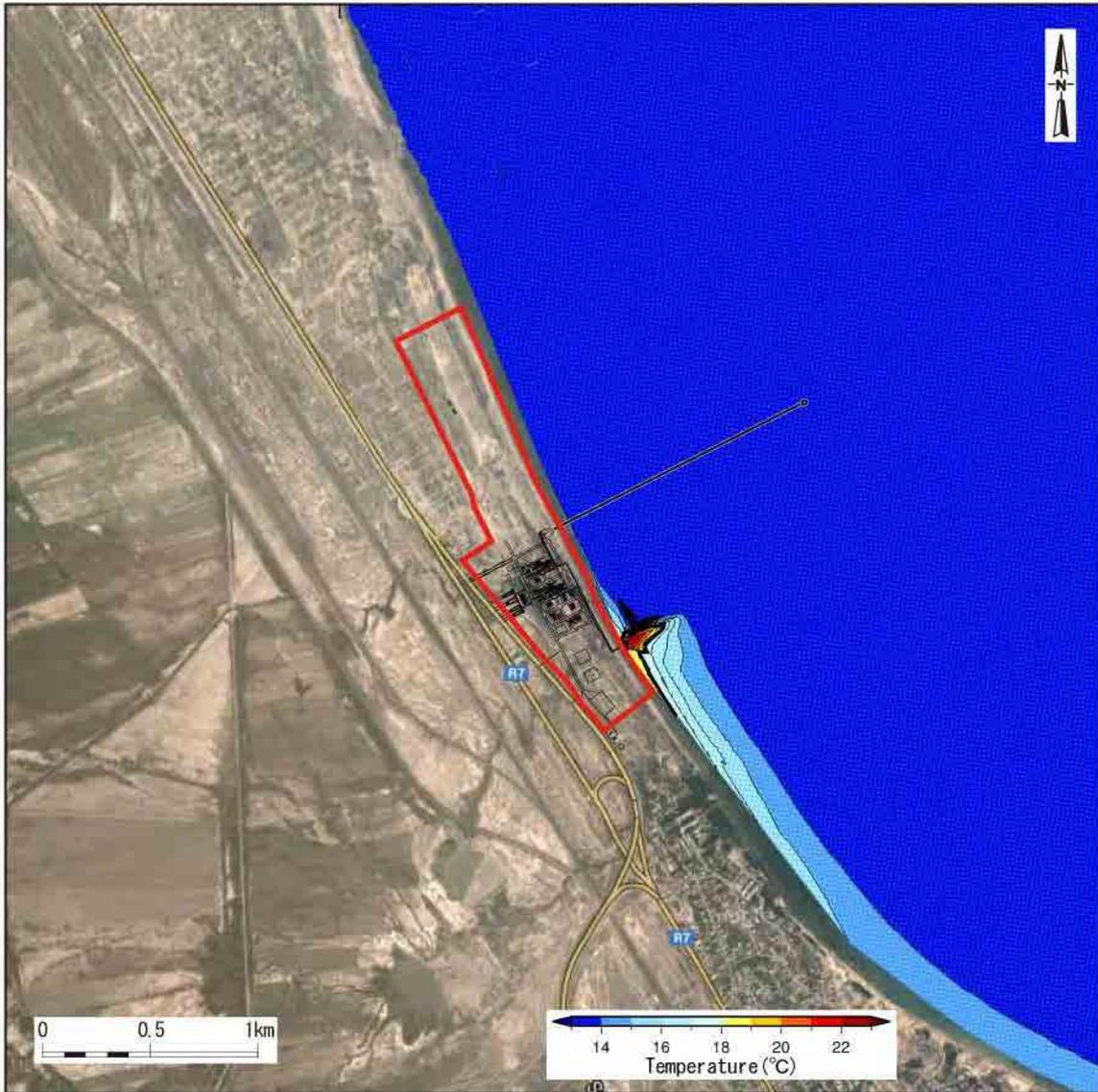
**Figure 13.6-13(1) Dispersion of Thermal Effluent (Current speed 0.3m/s: SE)**
