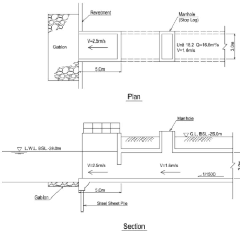
**Figure 13.6-11 Water Intake Structures**
