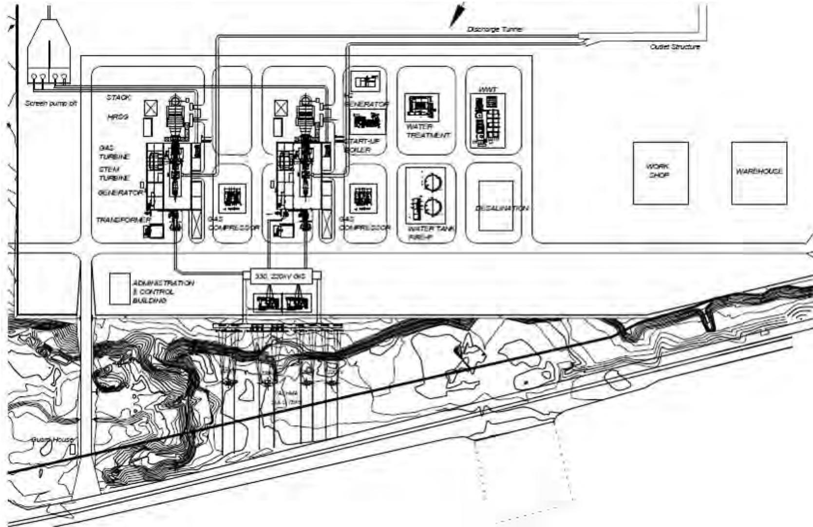
Figure 13.1-2 Conceptual Site Layout for the New Plant
