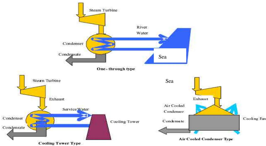
**Figure 13.3-3 Three Method of Cooling System**
