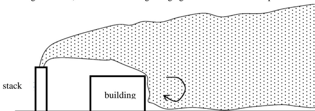
Figure 13.6-4 Diagram of Downdraft
