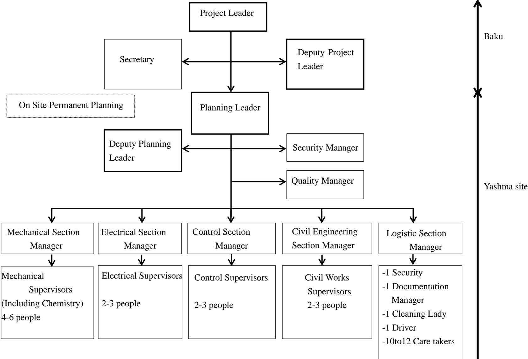
Figure 11.1-1 Organization Chart for the Construction Stage
