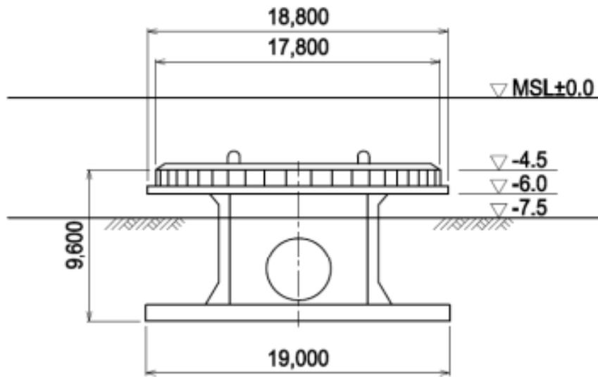
**Figure 13.6-10 Water Intake Structures**
