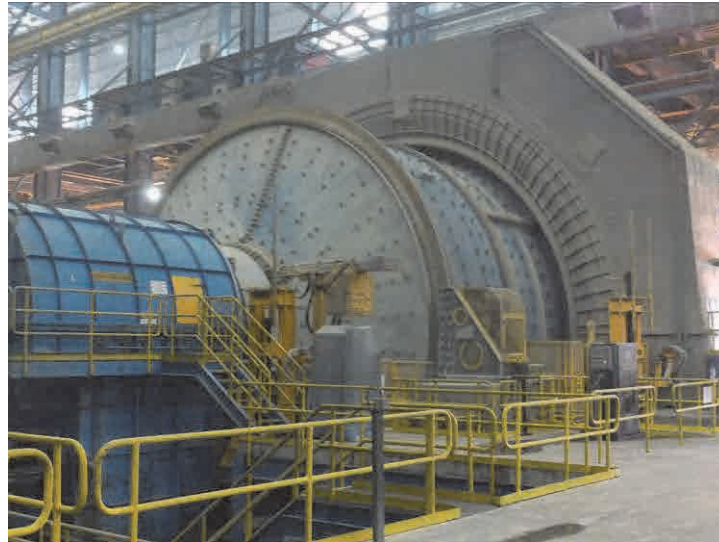
Photo 2.2.5 Ore Grinding System in Concentrator of Oyu Tolgoi Mine
