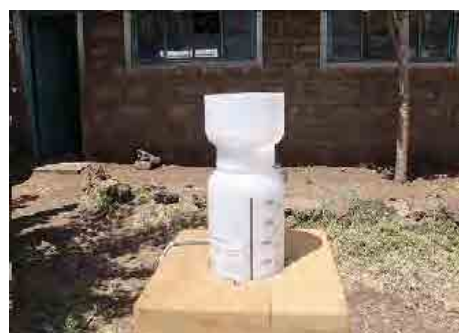
Simple Rain Gauge (Place: Nkando Primary School)
