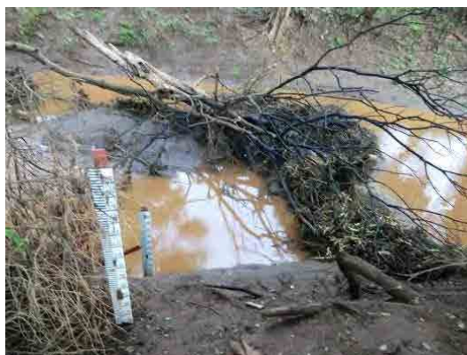
Water Level Gauging Station No. : 3J15 Measure water level of Lumi River.
