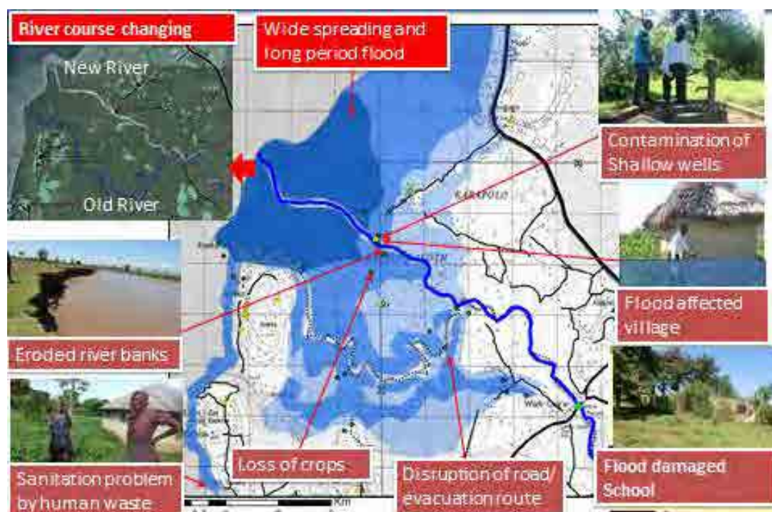
Figure 3.2.3 Flood Characteristics in the Low-lying area of Lower Gucha Migori River
