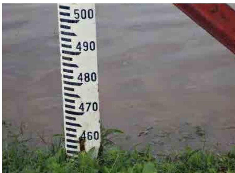
Figure-16 Water Level Gauge (unit: mm)
