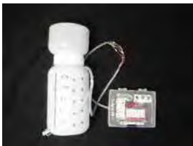
Figure-24 Convenient Rain Gauge and its Monitoring Instrument
