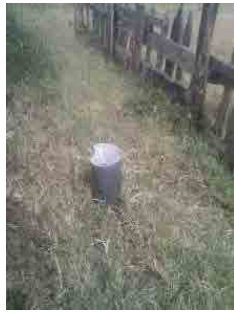
Broken Rain Gauge
