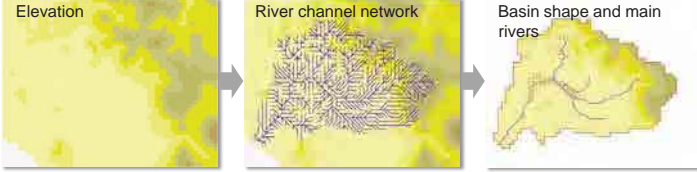
Basin boundary made from elevation Basin boundary from shapefile Solo river basin, Indonesia
