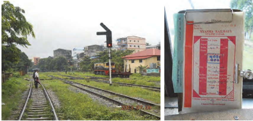
Figure 2.2.2.6 Current Automatic Block Color light Signal and Paper Token System
