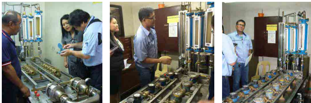
Pict-3.2.6 Water meter test laboratory: Before installation (Left), During measurement (Center, Right) [3-13]
