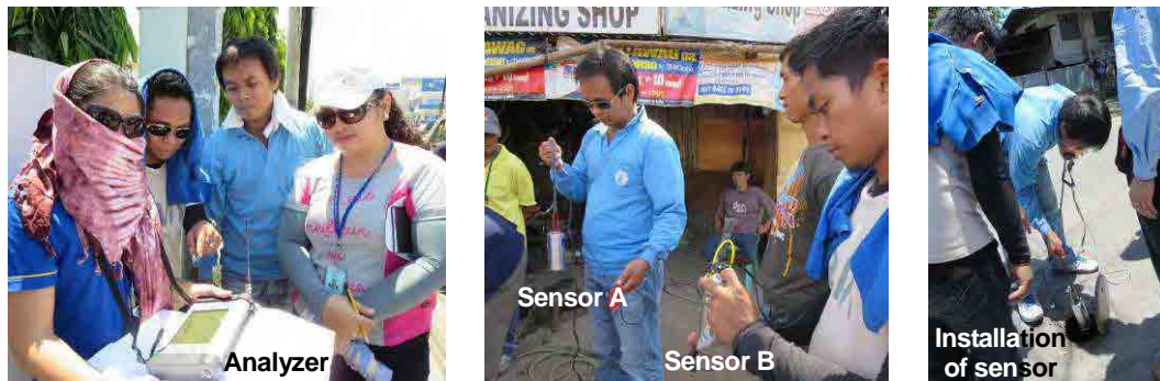
Pict-3.5.1 Water leakage survey by AQUASCAN 610
