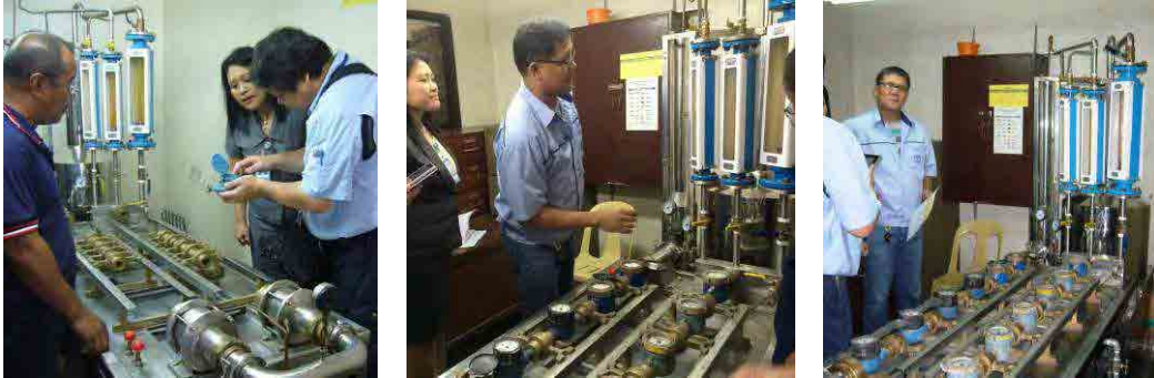
Pict-3.2.6 Water meter test laboratory: Before installation (Left), During measurement (Center, Right)
