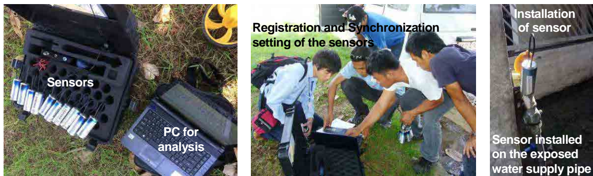
Pict-3.5.2 Water leakage survey by ZONSCAN 820
