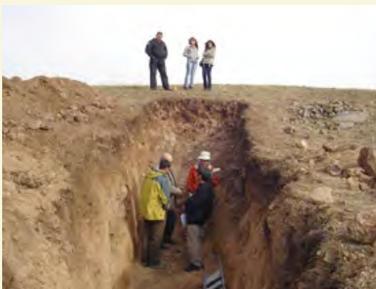
Trench survey technology, to study active faults, is transferred to the members of the National Survey for Seismic Protection.
