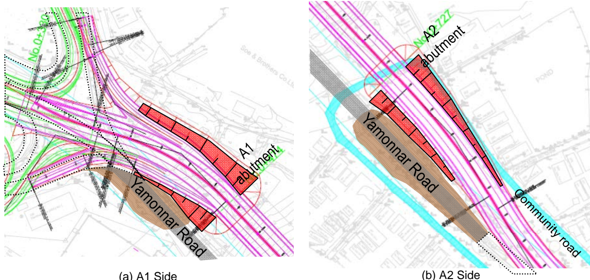
Figure 2.3.3 Areas Affected by Embankment Slopes
