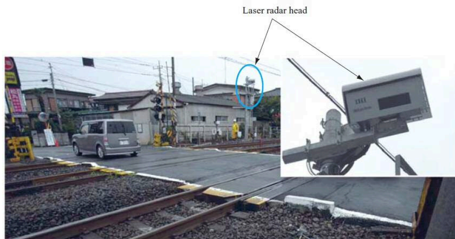
Source: http://www.ihl.co.jp/3DLaserRadar/en/pdf/3dlr_2008.pdf [Fig. 8-4-8] Japanese 3D Laser Radar Obstacle Detector
