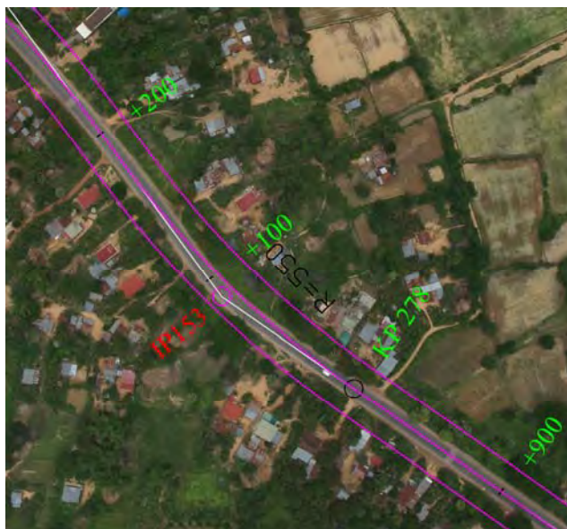
Figure 8.2-3 Proposed Alignment at KP 277 + 996 – KP 278 + 179 (IP153) (Radius of existing curve is 121m: Proposed to improve to radius of 550m)
