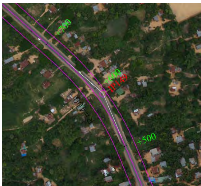
Figure 8.2-2 Proposed Alignment at KP 276 + 498 – KP 276 + 676 (IP149) (Radius of the existing curve is 155m: Proposed to improve to radius of 400m)
