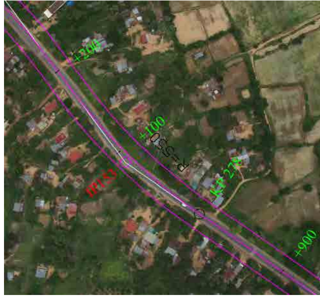
Figure 8.2-3 Proposed Alignment at KP 277 + 996 – KP 278 + 179 (IP153) (Radius of existing curve is 121 m: Proposed to improve to radius of 550 m)
