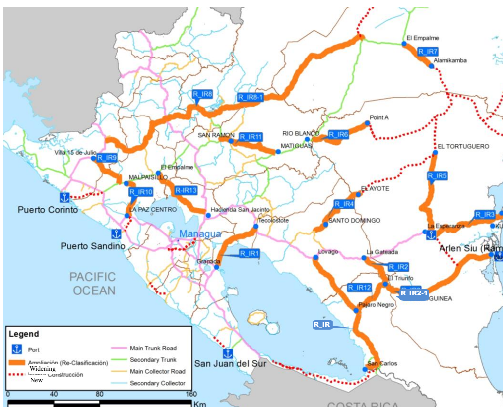
Figure 16.1.15 Proposed Roads for Rehabilitation
