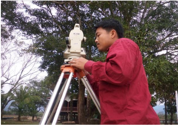
ວັດແທກດ້ວຍກ້ອງມູມ (Measurements by Total Station)
