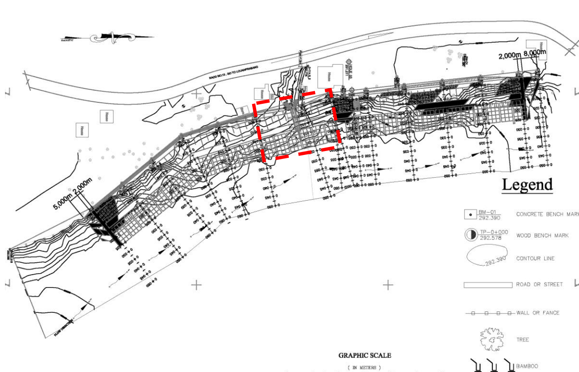
Fig. 3.4-7 Layout of Riverbank Protection Works at Souanlouang (Nasa) Site (Additional Works Including Confluence Between Small Stream and Khan River, Total Length: 40m)
