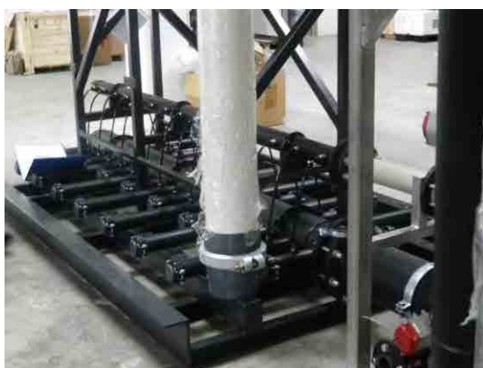
Figure 3-2 One Unit of UF
