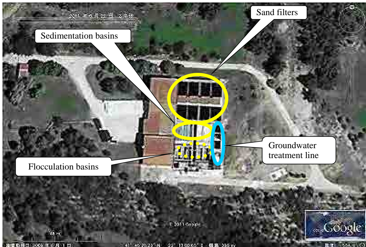
Figure 2-4 Existing Stip WTP Layout
