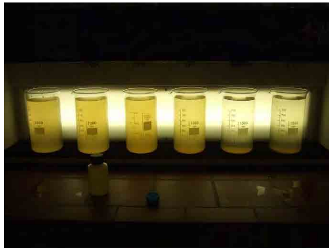
Figure 3-10 Jar Test to Identify the Chemical Dosage Rate
