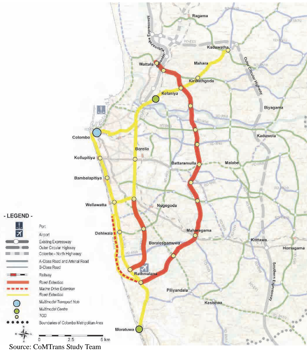
Figure 5.13.11 Road Development for BRT Operation
