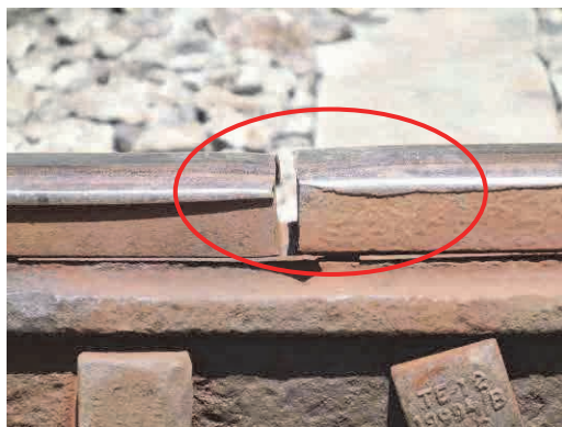
Figure 3.2.11 Deformation of Rail
