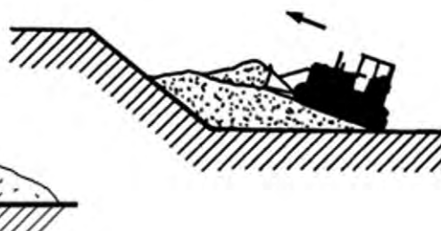
Figure 3-5: Method of pushing the waste upwards
