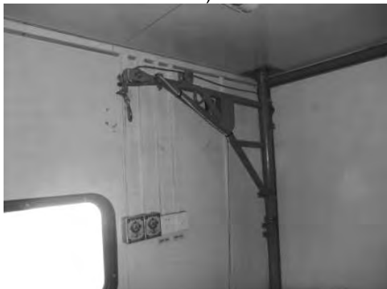
Electric-powered crane (rotary jib stretches out)
