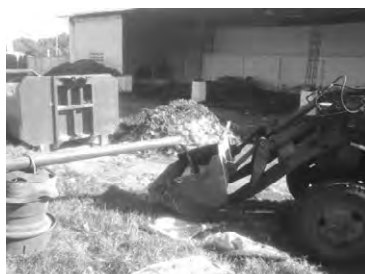
Photo 1-30: The wheel loader receiving fermentation liquid from the anaerobic fermentation tank
