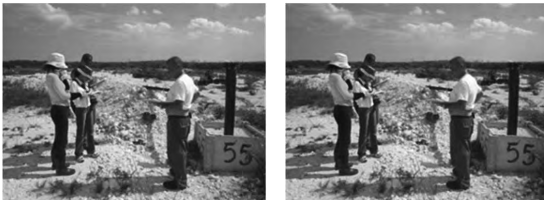
Photo 3-15: Height measurement using simple GPS
