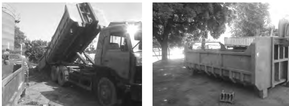
Photo 1-46: Arm roll typed truck and large sized containers (20m 3 )
