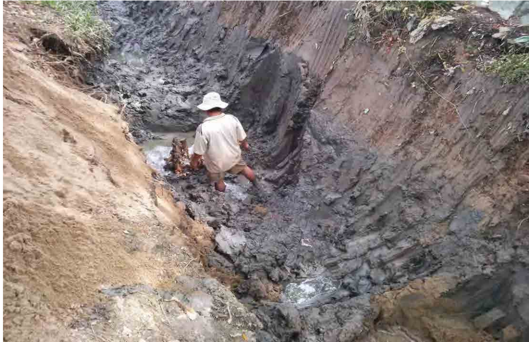
Photo2 : The weak clay mud layer in drainage ditches near the Site A02
