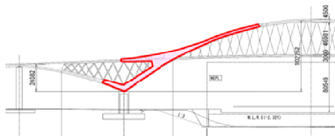
Figure 20.7 Components using SBHS in the Project (Main Bridge of the 4th Panama Canal Bridge)
