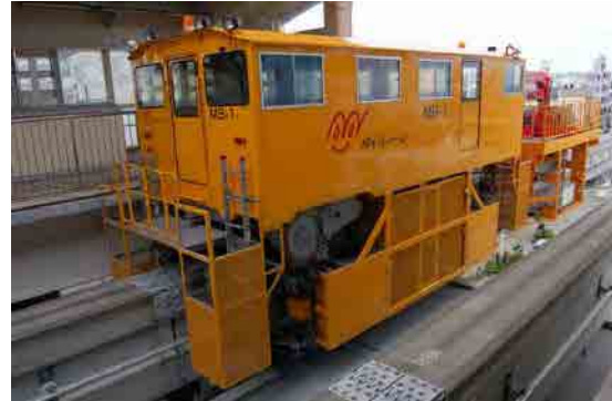
Mobile Work-Shop (Coupled with Crane Car) [ Okinawa Urban Monorail ]
