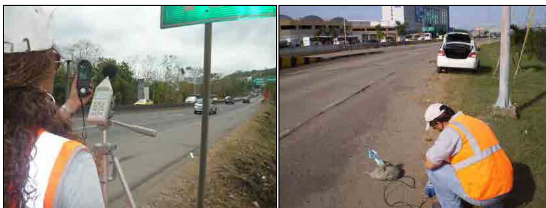
Figure 19.5 Noise (L) and Vibration (R) Surveys
