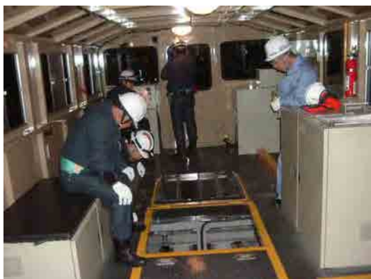
Inside Mobile Work-Shop (Visual Inspection of Track) [ Okinawa Urban Monorail ]
