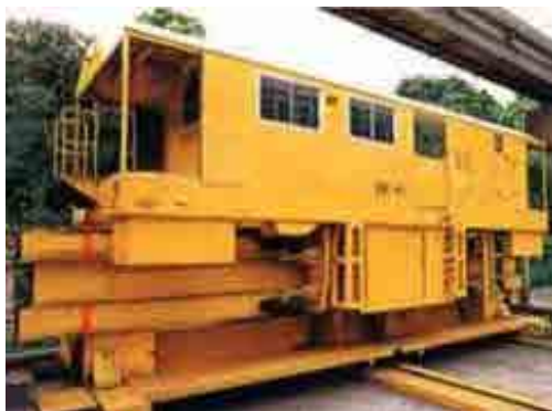
Mobile Work-Shop (Diesel Engine) [ Tokyo Monorail ]
