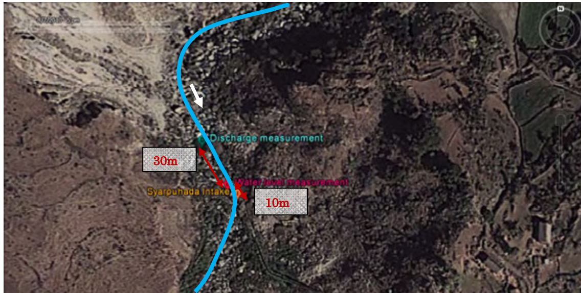
Figure 1.6 Location of Discharge Monitoring (Syarpudaha)
