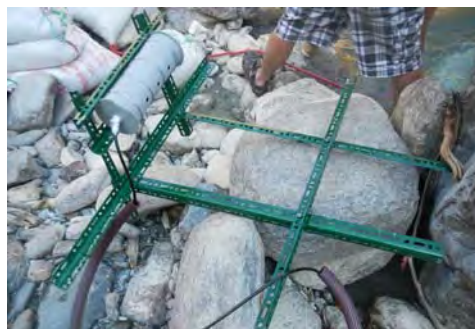
Figure 1.1 Water Level Gauge with Foundation
