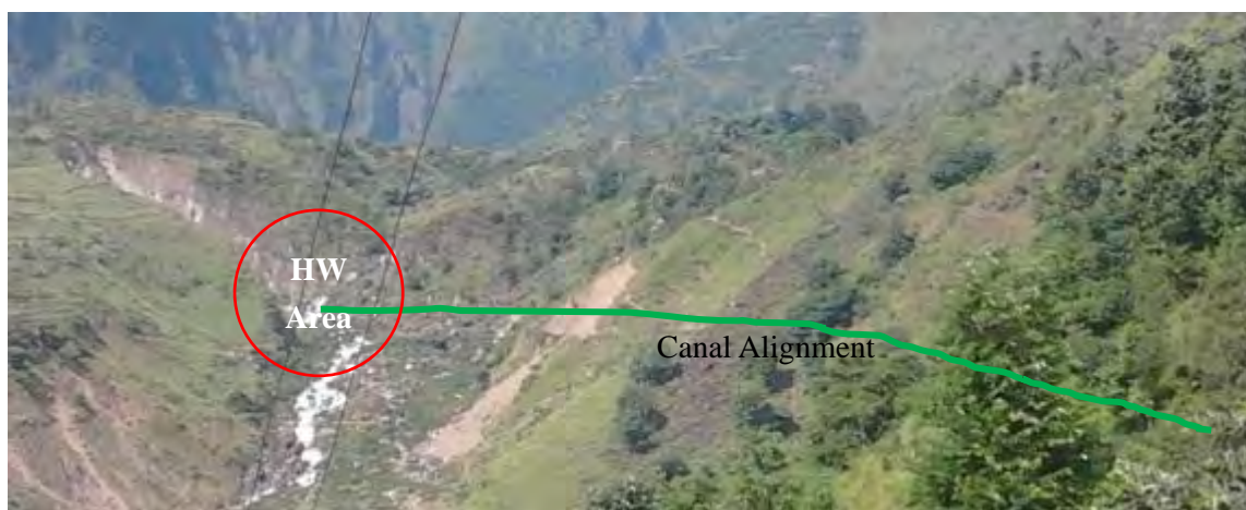
Figure 7-27 Headworks Location and Canal Alignment
