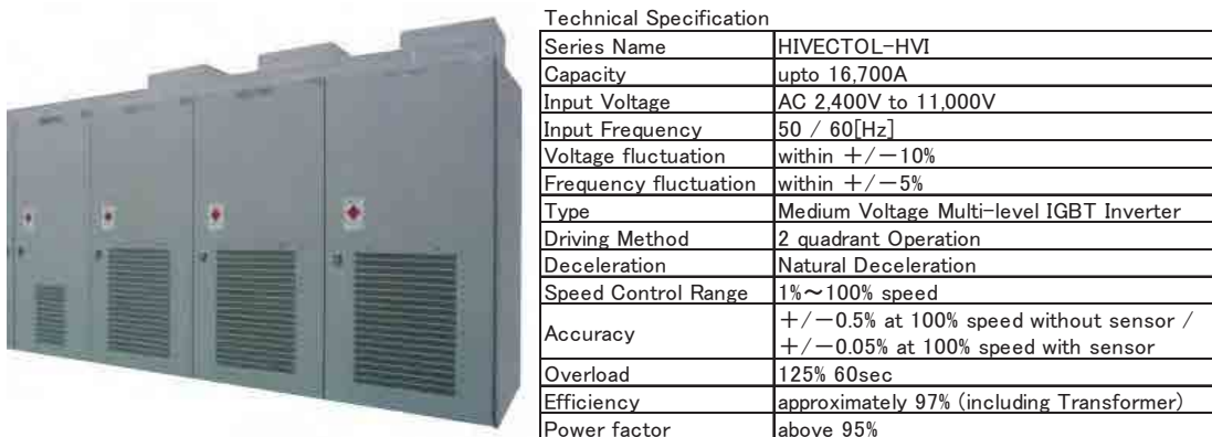
Figure 3-4-5 Example of a high efficiency inverter
