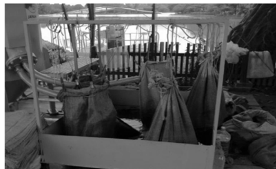
Algae Collection Jute Bag & Stand To dehydrate and collect by Jute Bag
