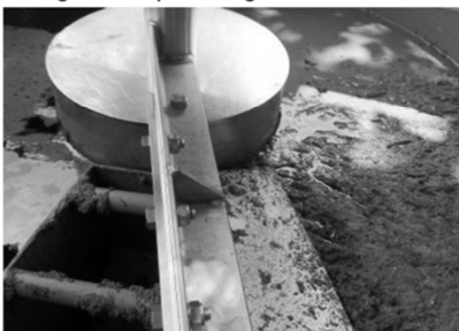
Algae Scraper To scrape and collect floating algae floc
