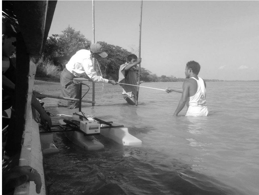
Discharge Measured by River Surveyor M 9 at Toe River
