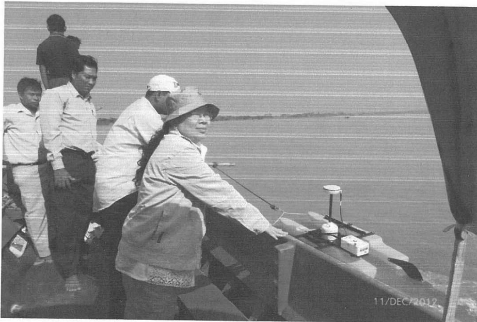
Discharge Measured by River Surveyor M 9 at Toe River
