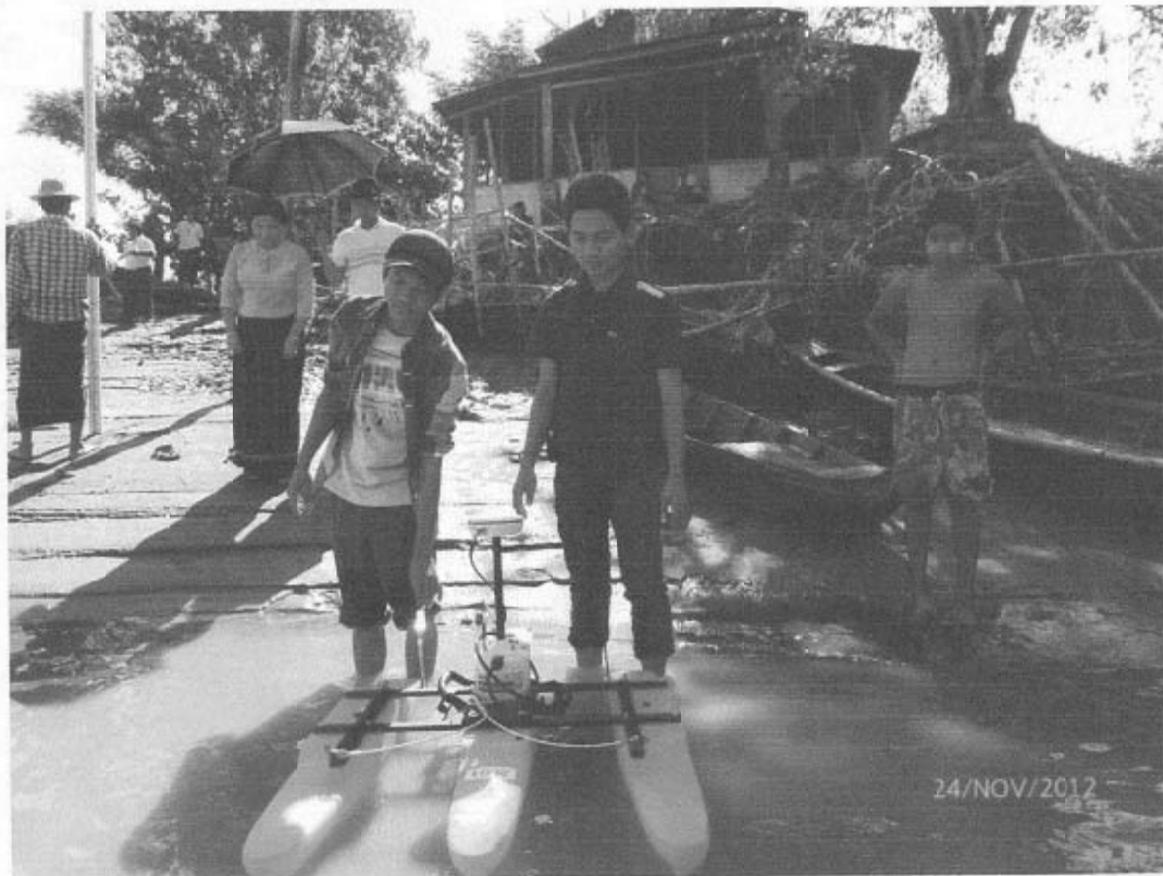
Preparing to measure Discharge by River Surveyor M9 at Kokkwa River
