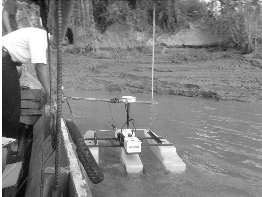
Discharge Measured by River Surveyor M 9 at Kokkowa River
