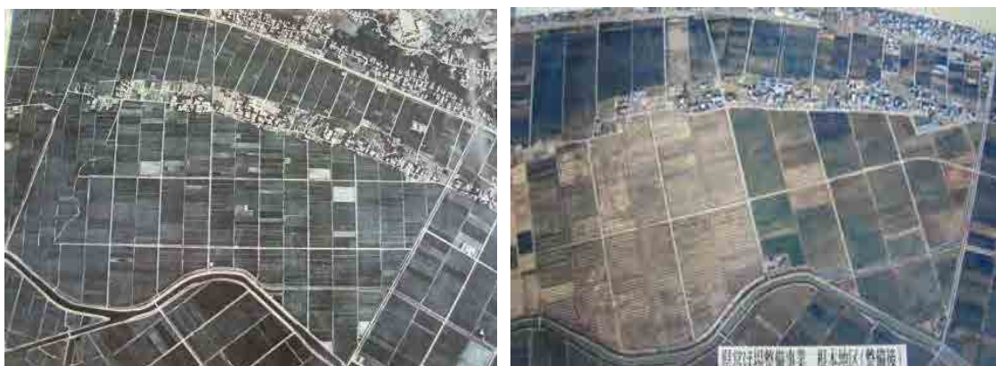
Figure 2.2.3 Farm Plot Size Enlargement from 0.2ha (left) to over 1ha (right) in Ibaraki, Japan
