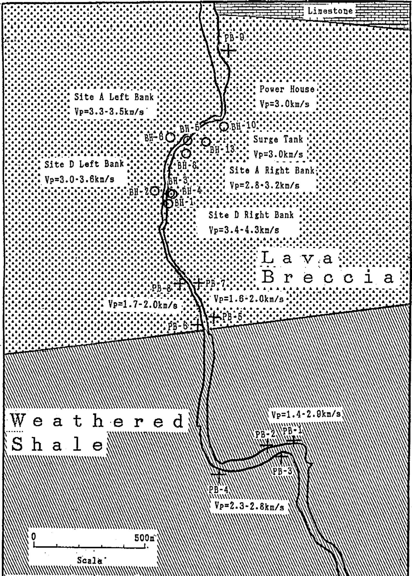
Figure 3-10 Geological Map Around Site with Seismic Wave Velocity of Base Rocks
