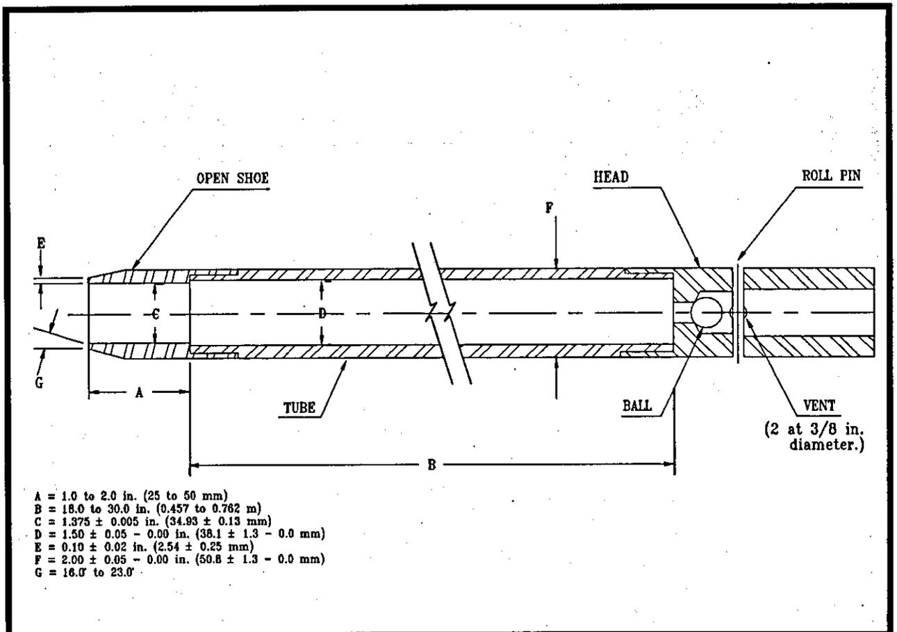
Figure A.2.1 Standard Penetration Split Barrel Sampler
