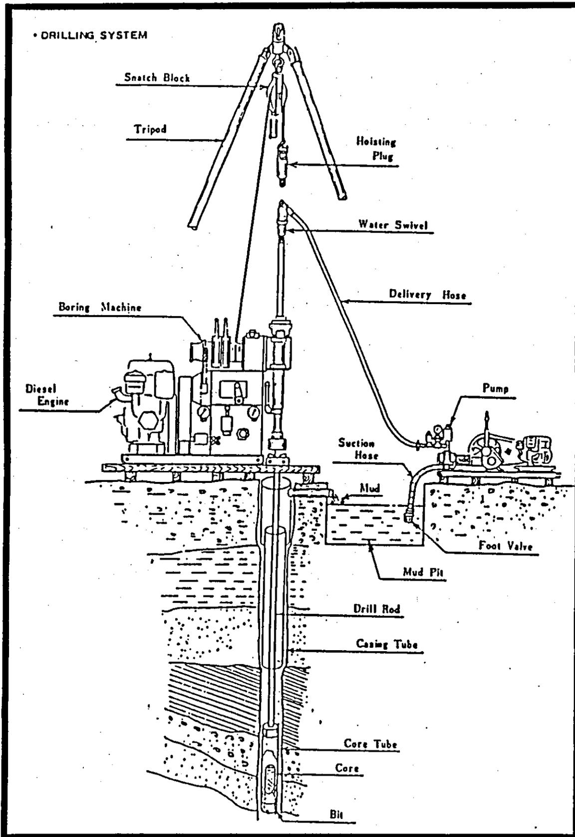
Figure A.1.1 Set up of Drilling Operation
