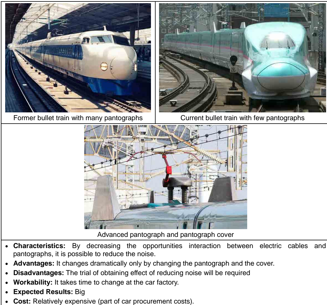
Figure 5.2.6 Example of Low-Noise Type Pantograph and Reduction of its Number
