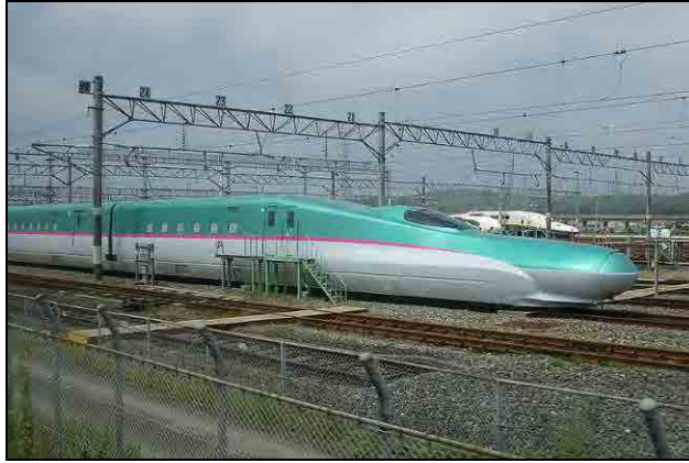
Figure 5.3.38 Long Nose Shape of Series E5
