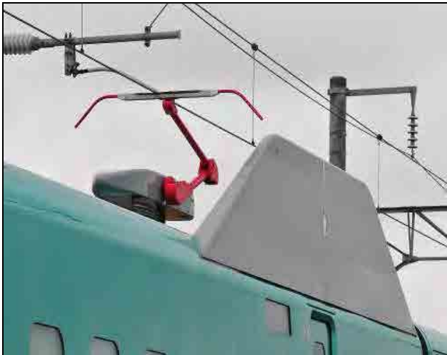
Figure 5.3.39 Low-noise Pantograph and Noise Reduction Plates
