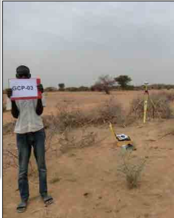
Ground control point pricking work (GCP03)
