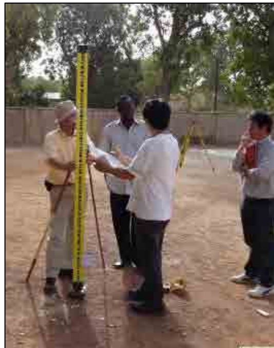
Photo 4-3 Instruction on installing a barcode leveling staff
