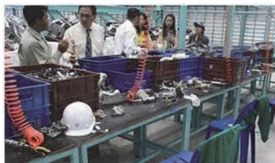
Manual dismantling line of E-waste
