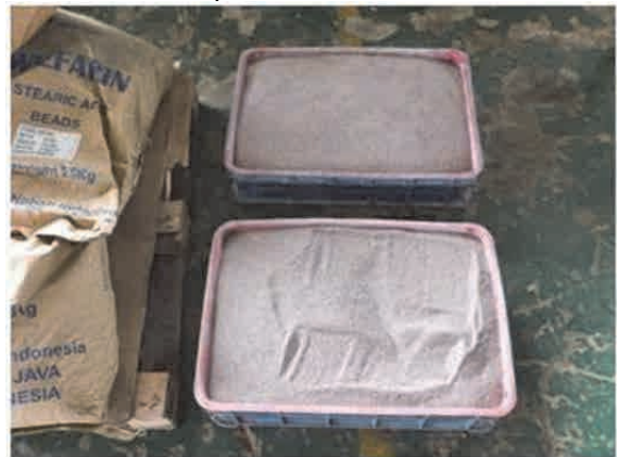
Powder containing copper after gravity separation (sellout as final product)
