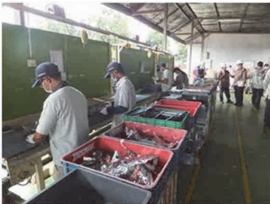
Manual dismantling of PCs and servers (PCBs are removed)
