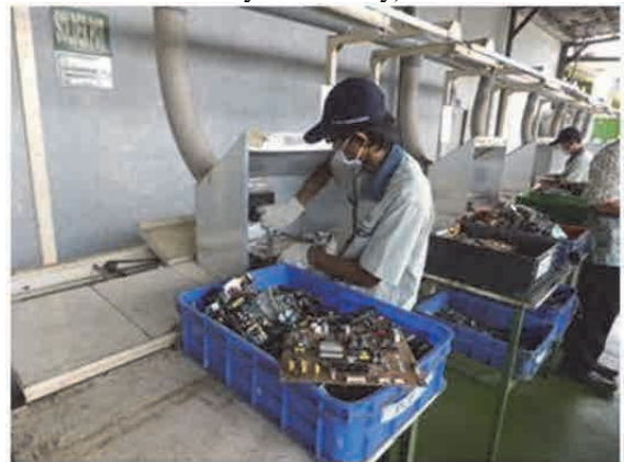
Melting solder to remove parts or components from PCBs
