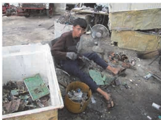
Manual dismantling with no protection
