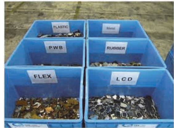
Parts and materials separated after dismantling
