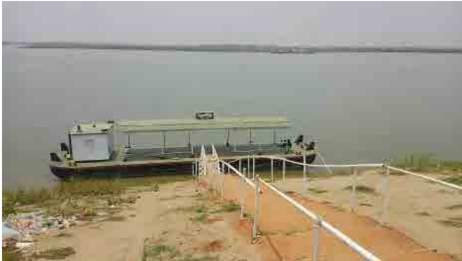
Large ships cannot dock because of shallow river bed. Instead passengers embark on ships by using the barge
