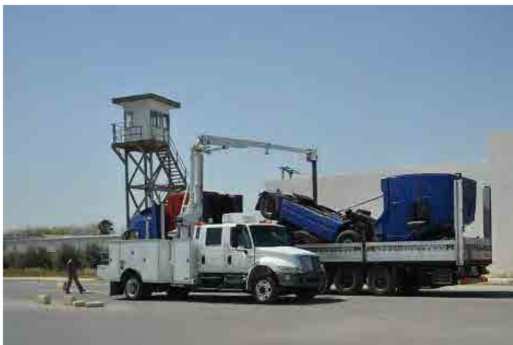
Figure 4.2-6 Inspection work with Mobile Scanner in SHB
